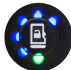
To lock or unlock SD card, quickly press SD lock button.
