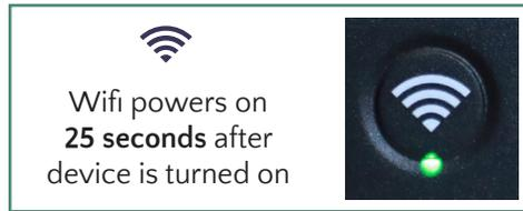
To power Wifi on/off, hold SD lock button for 2 seconds
