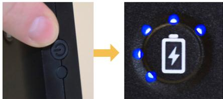
To Charge a Phone: Plug the phone into the USB port and tap the power button.
